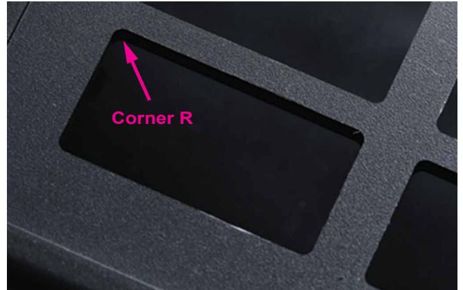
All milling with corners / edges shall have a standard R1.0 radius (smallest R0.5 radius possible).
