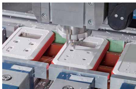
7. Machining on enclosure
