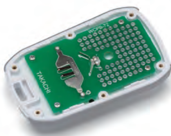
Install the PCB in the top cover
