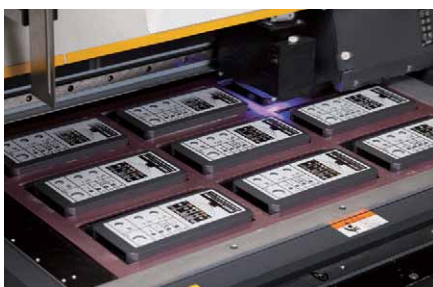
Digital printed overlay
