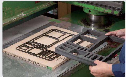
For mass production, cost-effective mold press cutting is also available.
