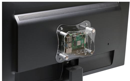
RPA-4B-1F is compatible with VESA Mount Standards (100 x 100mm), and can be installed on the back side of PC displays, etc.
