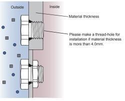
If used with a lock nut, material thickness should not exceed 4.0mm.
