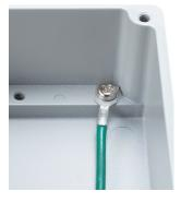
When tightened, protrusions on the underside of the screw head will shave away at the painted or anodized surface to expose the base material for achieving conductivity.
