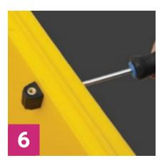
Tighten the screw firmly. (Recommended torque :  $0.8 \sim 1.0 \text{ N} \cdot \text{m}$ )
