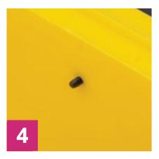
After the hole is drilled, insert the screw from the exterior side.
