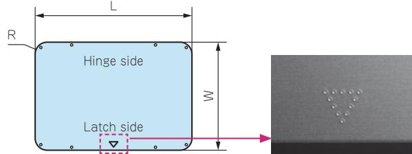
※Install panel with ▽ marking towards the latch.
