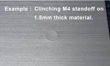
Example : Clinching M4 standoff on 1.5mm thick material.
