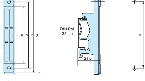
Installed on 35mm DIN-Rail
